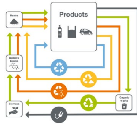
Material flow model with a focus on different end-of-life solutions. Some material loss occurs at all product life cycle stages and should be replenished with renewable resources.
